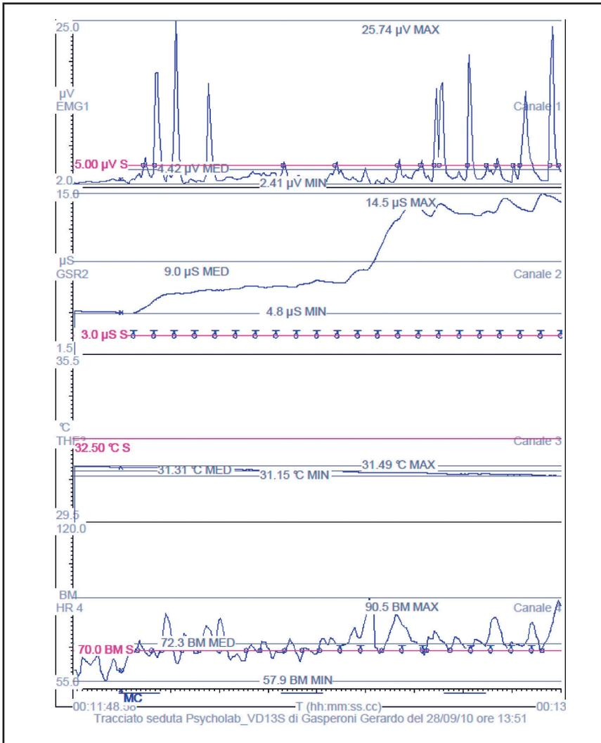
Fig. 1. On line display of the psychophysiological trend. On the first stripe Electromiogram (EMG) measured in  $\mu\text{V}$ ; on the second one, skin conductance in  $\mu\text{S}$ ; on the third peripheral temperature in Celsius and on the fourth the heart rate. At the bottom, MC means the start point of the stressor, i.e. mental subtraction.
